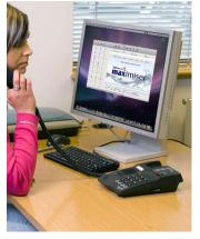
IP Phone, designed to work with **max**imiser to address everyday business telephony needs. The PCS 520 is a display phone with pre-configured system access keys, desktop paging and combined Do No Disturb/Message Waiting LED, with the entry-level PCS 505 completing the range.
