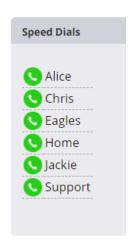
Your Speed Dials will be displayed within the Web Phone page within the Speed Dials list on the right hand side. They can be used to quickly and easily make calls, transfer calls and pick up calls.
