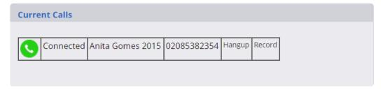
If the number dialled is matched in the telephone system's directories the Contact's or User's name will also be displayed within Current calls.
